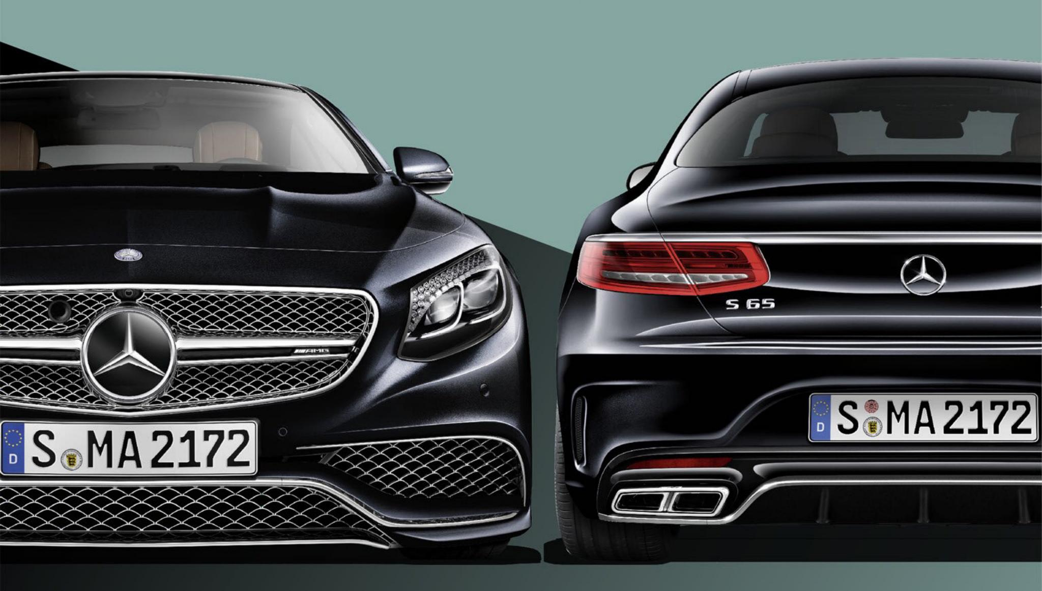
The three-dimensional front splitter reduces lift at the front axle, while the gap above the front splitter ensures an effective flow of air to the separate engine oil cooler behind it.
